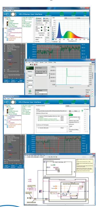
HELIOSense Software is the primary interface for HELIOS components and systems. It is a flexible architecture where any hardware built into the Labsphere API (LSAPI) can be recognized and used in HELIOS systems.
